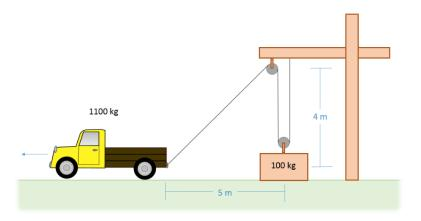
(Solution: distance traveled = 6.7 m, truck speed = 2.12 m/s, work done: 5464.92 J)
