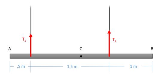
(Solution:  $a_{cy} = .5 m/s^2$ ,  $\alpha = .333 rad/s^2$ ,  $T_1 = 81.75 N$ ,  $T_2 = 176 N$ )
