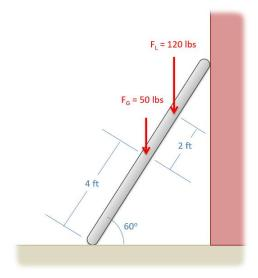
Solution:  $F_{N \text{ Top}} = 66.4 \text{ lbs}$ ,  $F_{N \text{ Bottom}} = 170 \text{ lbs}$ ,  $F_F = 66.4 \text{ lbs}$
