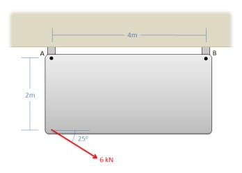
Solution:  $M_A = 10.88 \text{ kNm}$ ,  $M_B = 21.02 \text{ kNm}$
