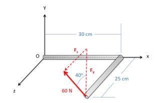
Solution:  $M_0 = [-11.49, -11.57, 13.79] \text{ Nm}, |M| = 21.36 \text{ Nm}$
