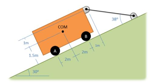
Solution: T = 21786 N,  $F_A = 7222 \text{ N}$ ,  $F_B = 35925 \text{ N}$
