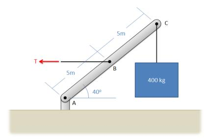
Solution:  $F_{AX} = 9352.9 \text{ N}$ ,  $F_{AY} = 3924 \text{ N}$ ,  $T_B = 9352.9 \text{ N}$
