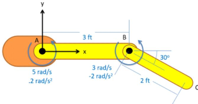
$$\begin{aligned}\theta_A &= 0^\circ \\ \dot{\theta}_A &= 5 \text{ rad/s} \\ \ddot{\theta}_A &= 2 \text{ rad/s}^2\end{aligned}$$
