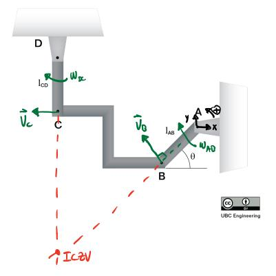
$$\vec{V}_{B} = \vec{W}_{AB} \times \vec{\Gamma}_{B/A} = -3\hat{\kappa} \times (-0.5\cos 45\hat{\gamma} - 0.5\sin 45\hat{\gamma})$$
